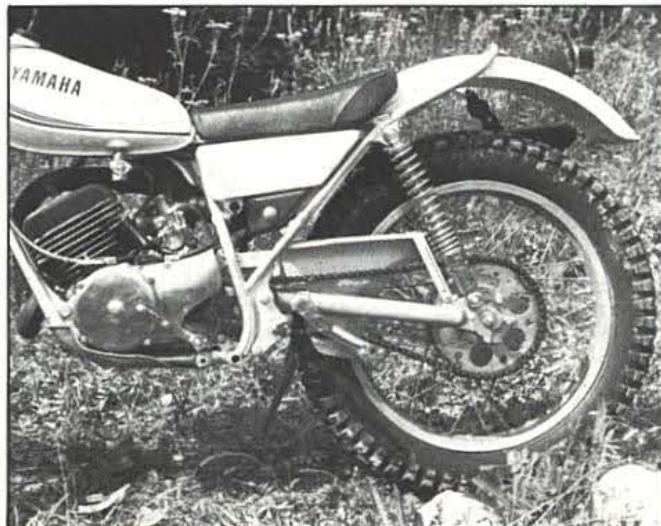
The back end of the Yam is too soft and the Dunlop doesn't grip like the Pirelli.
