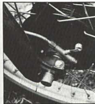
Front brake is good and speedo drive is adapted from the XL.
