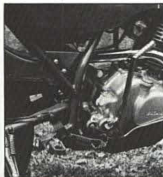
Rear brake is a bit close to kick start shaft.
