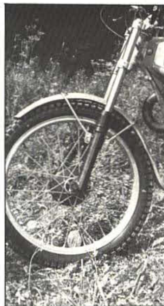
The Bully's fork works well and the brake has a chromed alloy hub.
