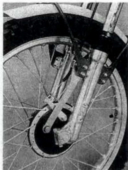
SWM introduced the first 38mm fork on the Jumbo. It's built for them by Betor.
