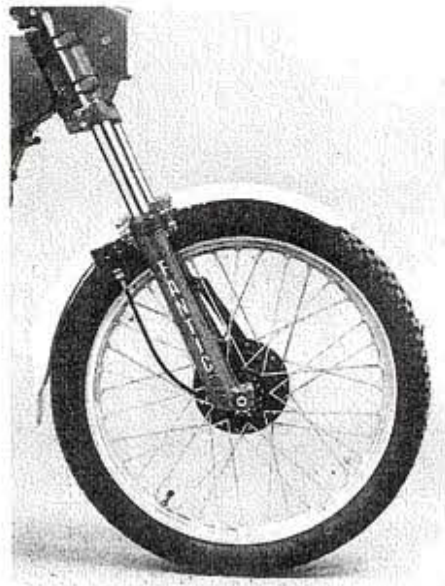
Leading axle fork on the Fantic is manufactured by Marzocchi.
