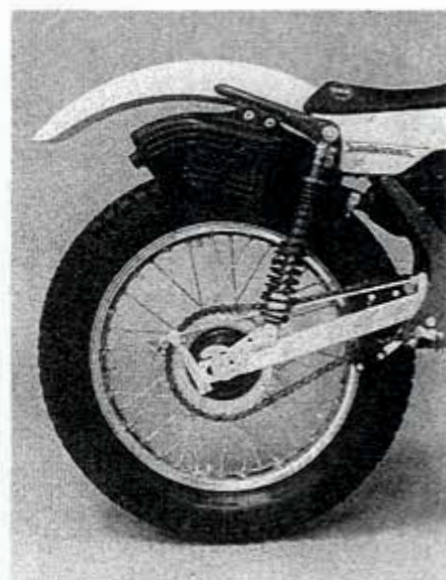
SWM fits Betor gas shocks on the Jumbo. The aluminum swingarm is a production first.
