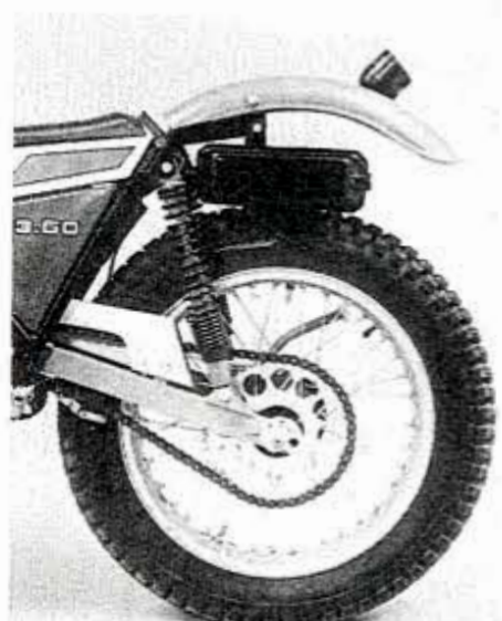
Betor shocks, traditionally favored by Spanish manufacturers, are found on the Cagiva.
