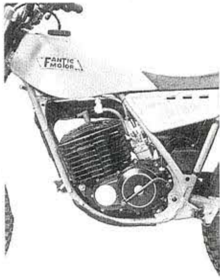
Fantic's 212cc motor produces exceptional power for its size. Compression is 11.7:1.
