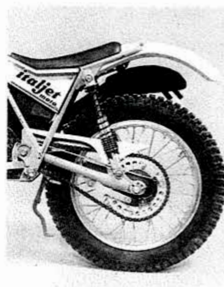
The Italjet's seat height tied for lowest of the five test bikes. Shocks are by Marzocchi.
